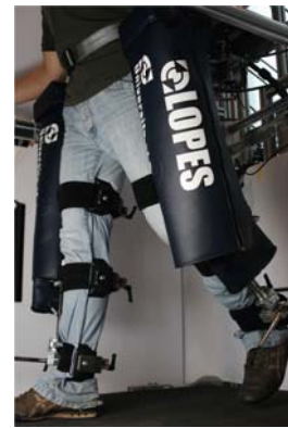
Figure 1. LOPES is an bilateral exoskeleton with the actuators detached from the exoskeleton. Series elastic joints are actuated via Bowden cables. LOPES has eight degrees of freedom that are impedance controlled.
